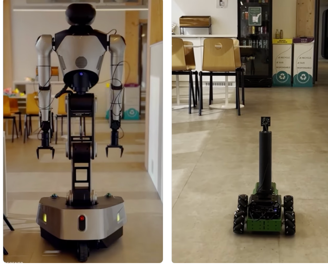
Figure 2: Cross-robot deployment of Robostrail Navigate on the Galaxea R1 (left) and Hiwonder JetAuto (right). The two platforms differ substantially in robot morphology, camera height, camera configuration, and base geometry. Both deployments use the same Robostrail Navigate vision-language model and diffusion policy weights, with only the low-level platform controller differing between robots.
