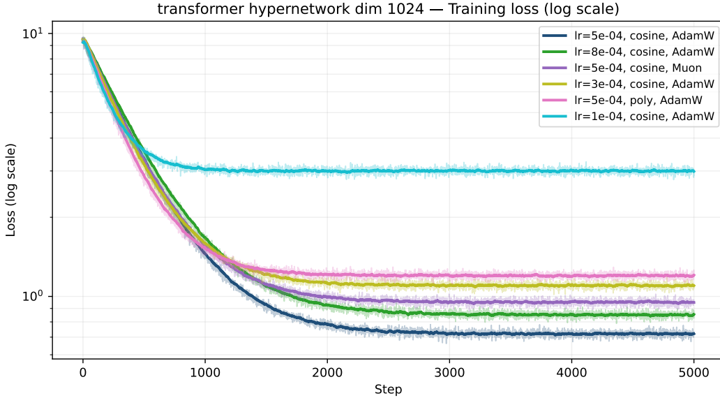
FIGURE 9: Hyperparameter sweep results for the largest width configuration ( d_{\text{model}} = 1024 ), showing training loss on a log scale across different learning rates, schedulers, and optimizers on a small-scale subset. Cosine annealing with AdamW with learning rate 5 \times 10^{-4} achieves the lowest final training loss, motivating its selection for all scaling experiments.
