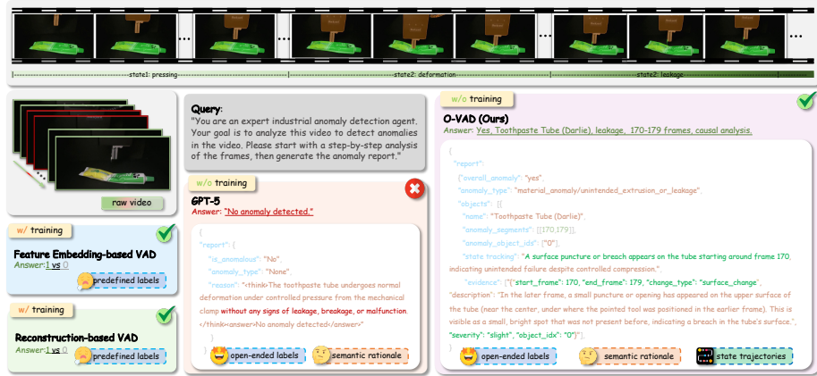
Fig. 1: Why object state evolution matters for industrial anomaly detection. The toothpaste tube undergoes pressing and deformation before a subtle leakage emerges. Traditional methods predict binary classifications. VLM prompting fails to detect it due to the lack of evidence. O-VAD tracks object-wise state changes and produces an open-ended anomaly report with in-depth analysis.
