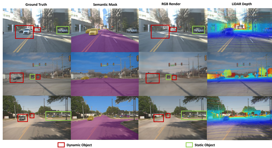
Fig. 3: Semantic masks for region-aware reconstruction. We generate ground, sky, and dynamic-object masks to support road regularization, sky modeling, and moving-object filtering, respectively. For movable categories, 3D tracking cuboids distinguish truly dynamic objects from stationary instances: red boxes indicate objects masked out, while green boxes indicate stationary objects preserved for reconstruction.
