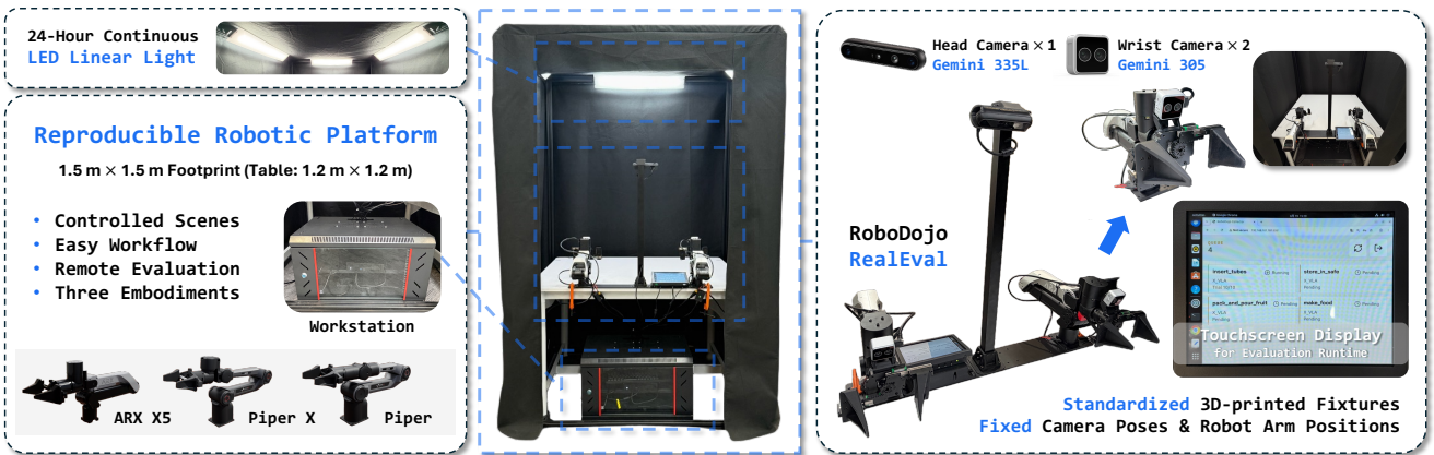
Figure 7: Overview of the RoboDojo-RealEval system. RoboDojo-RealEval provides a standardized physical platform for reproducible real-world robot manipulation evaluation, with controlled workspace geometry, fixed robot and camera mounts, stable lighting, a touchscreen evaluation interface, and support for three collaborative bimanual embodiments.
