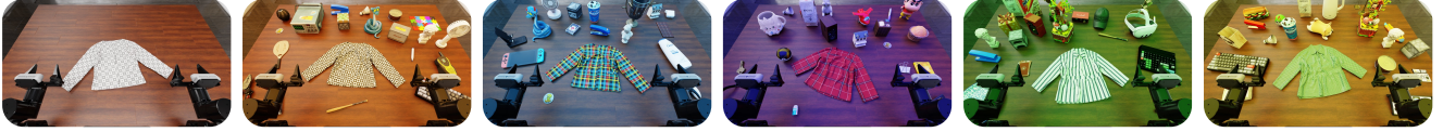
Figure 8: Domain randomization in RoboDojo. We visualize the effects of domain randomization in simulation, including variations in background, lighting, clutter layout, object appearance, and scene configuration. These randomized environments increase visual diversity and reduce overfitting to a fixed simulation setting.
