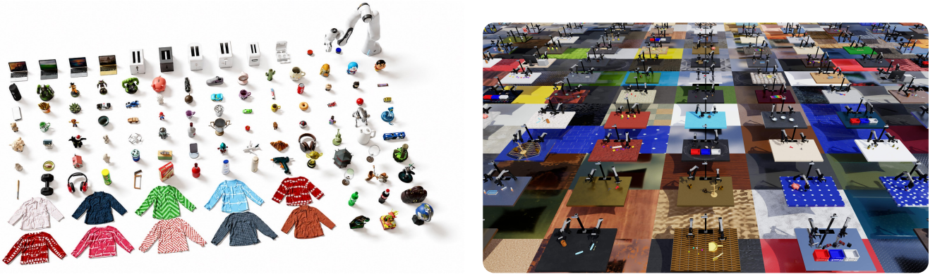
(a) Asset library. Sample rigid, articulated, and deformable assets. (b) Parallel simulation. Concurrent heterogeneous task execution.
