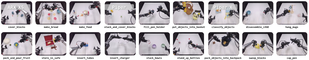
Figure 2: Task Overview of RoboDojo. RoboDojo includes 42 simulation tasks and 18 real-world tasks for evaluating generalist robot manipulation policies. The simulation tasks are organized into five capability dimensions: Generalization, Memory, Long-Horizon, Precision, and Open, enabling efficient capability-oriented diagnosis. The real-world tasks assess policy behavior under challenging and reproducible physical deployment conditions. Together, these tasks cover diverse manipulation skills, spatial configurations, and bimanual coordination patterns across simulation and the real world.
