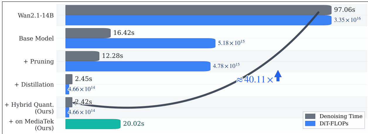
Figure 2 Denoising time and DiT-FLOPs comparison of CineMobile across different acceleration stages. Wan2.1-14B is used as the teacher model, requiring 97.06s denoising time and 3.35 \times 10^{16} DiT-FLOPs. Starting from the base model Wan2.1-v1.1-Fun-1.5B, pruning reduces the model complexity and brings a moderate speedup, reducing the denoising time from 16.42s to 12.28s. Distillation further enables 4-step generation, leading to the main efficiency improvement with 2.45s denoising time. After applying hybrid precision weight quantization, CineMobile achieves 40.11 \times faster DiT denoising and 71.89 \times lower DiT-FLOPs than the teacher model. On the MediaTek Dimensity 8400 Ultimate 5G platform, CineMobile achieves a per-step denoising latency of 20.02s.
