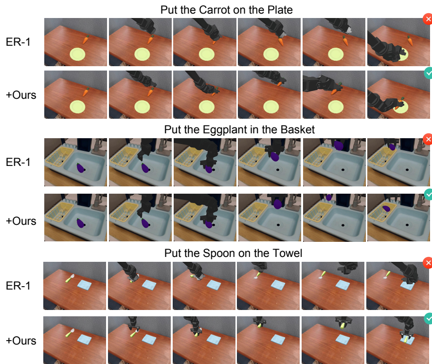
Fig. 9: Qualitative comparison between ER-1 and ER-1+Ours (E-TTS) on SimplerEnv on three manipulation tasks: “Put the Carrot on the Plate,” “Put the Eggplant in the Basket,” and “Put the Spoon on the Towel.” While ER-1 often fails to complete fine-grained placement due to inaccurate spatial reasoning, our E-TTS-enhanced model achieves more consistent object alignment and successful task completion.
